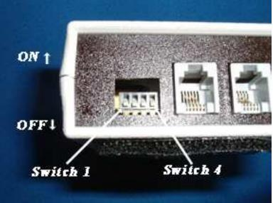
Most systems will use Straight Thru dial mode to send faxes. The DIP switches as shown in the above photo are set to Straight Thru dial mode, Normal Operating mode. In other words, the unit comes ready to control your fax immediately.
